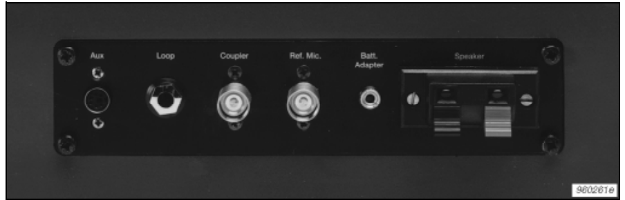
Fig. 1 Back panel of the Anechoic Test Box Type 4232. All connections to the inside of the test box are made via the connectors on the back panel
